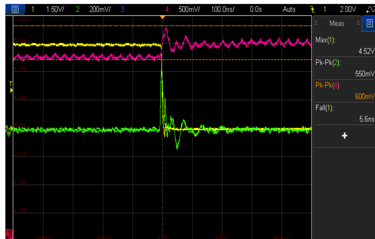
Figures 14 and 15: Shows the rise/fall times of Pin 13 (yellow waveform), shows the quiet high noise (pink waveform) and the ground bounce on quiet low (green waveform)
