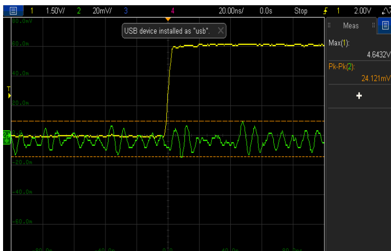
Figure 20 and 21: Shows the near field emissions on the Commercial Arduino
