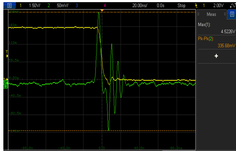
Figures 18 and 19: Shows the near field emissions on the Commercial Arduino
