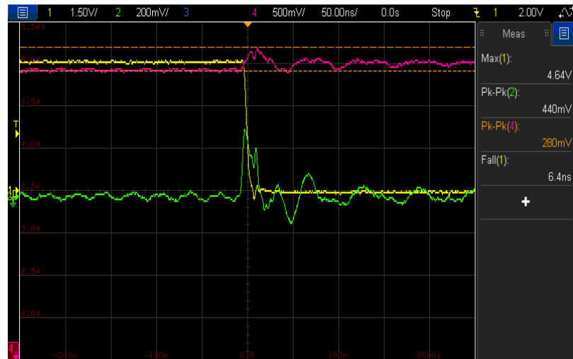
Figures 16 and 17: GOLDEN ARDUINO— Shows the rise/fall times of Pin 13 (yellow waveform), shows the quiet high noise (pink waveform) and the ground bounce on quiet low (green waveform)
