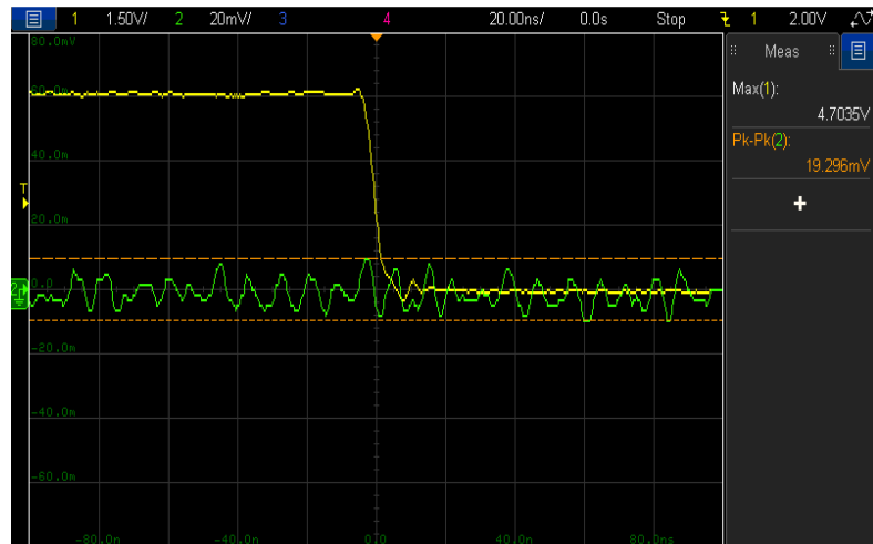
Figure 20 and 21: Shows the near field emissions on the Commercial Arduino
