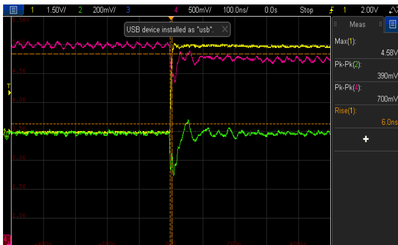
Figures 14 and 15: Shows the rise/fall times of Pin 13 (yellow waveform), shows the quiet high noise (pink waveform) and the ground bounce on quiet low (green waveform)
