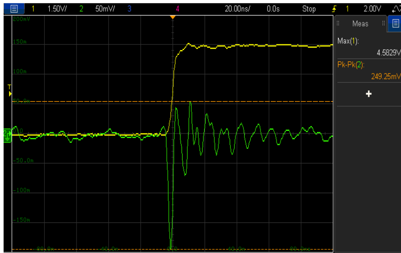
Figures 18 and 19: Shows the near field emissions on the Commercial Arduino
